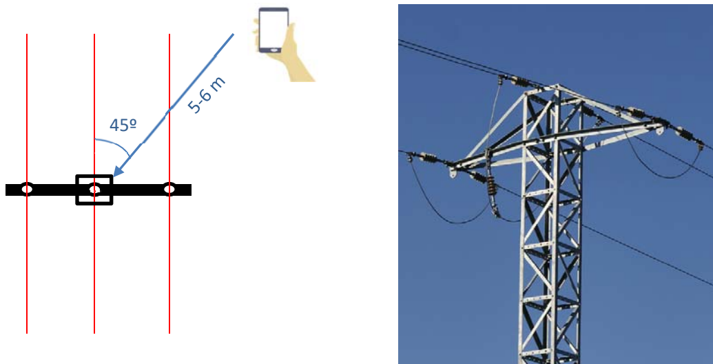
Figure 1. Position recommended for taking a photo of the pylon (aerial view, from above) on the left and expected result on the right.
